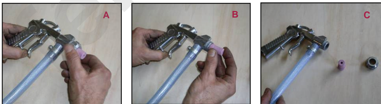
Figure 11 - Disassembly of the sandblast gun nozzle.
