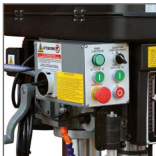
Panel de control
