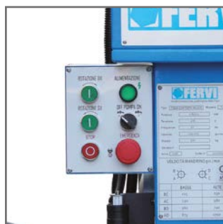
Panel de control
