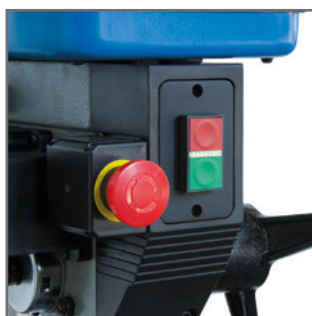
Panel de control
