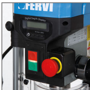
Panel de control
