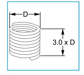
D Pack Packaging dimensions Gross weight EAN Code M 20 x 2.0 mm 10 -0,04 kg
