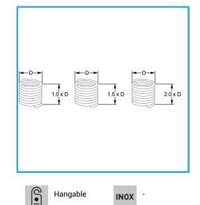
D Height Pack Gross weight EAN Code M 4 x 0.7 mm 1.5 D mm 25 0,00 kg 8012667368807
