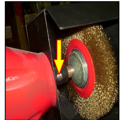
Figure 14 – Hole on the shaft.
