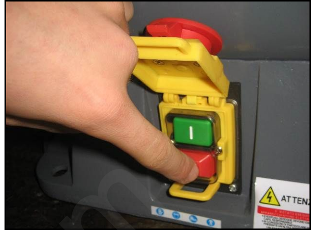
Figure 15 – Turning off the grinding wheel.
