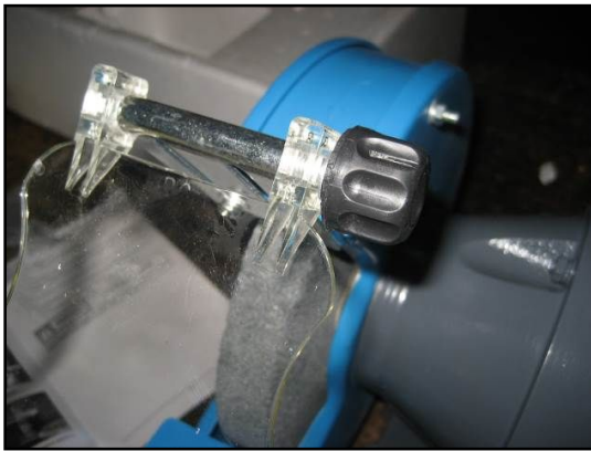
Figure 5 – Assembling the protective screens.
