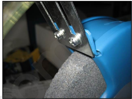
Figure 5 – Assembling the protective screens.
