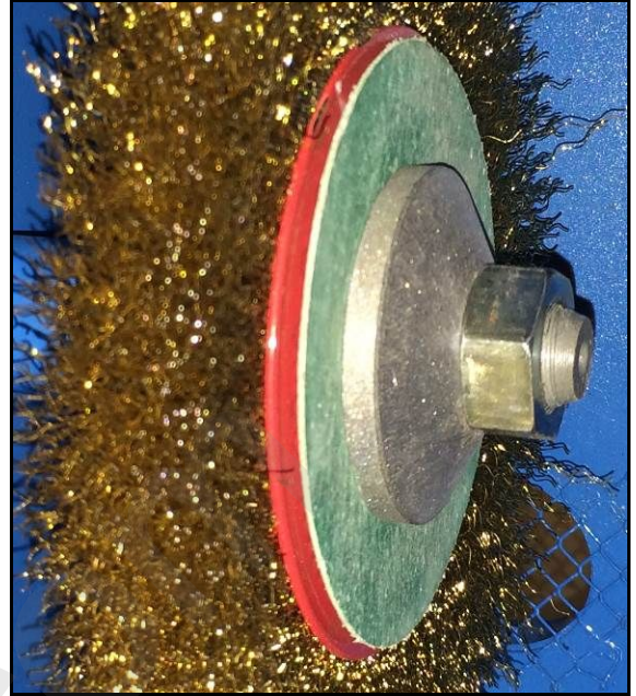
Figure 18 – Fastening nut and flange.
