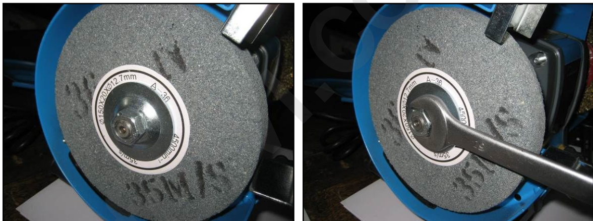
Figure 17 – Fastening nut and flange of the grinding wheel.
