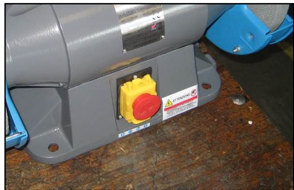
Figure 4 – Close-up of fastening holes.
