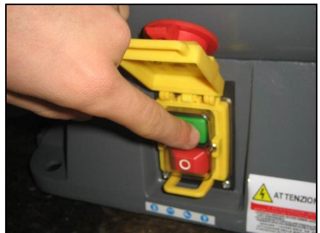
Figure 14 – Starting the grinding wheel.
