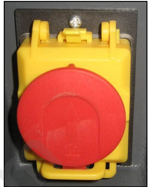
Figure 13 – Emergency stop button cap.
