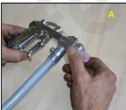
Figure 12 - Disassembly of the sandblast gun nozzle.
