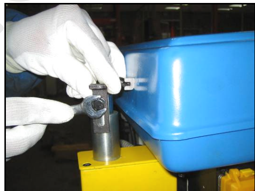
Figure 3 – Fitting and Adjusting the End of the Rod.
