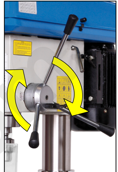
Figure 28 - Lowering the spindle.
