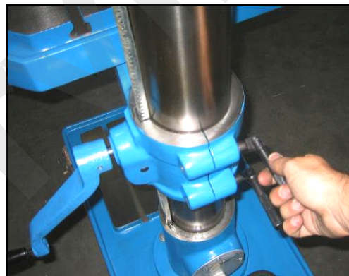
Figure 15 – Unlocking the screws.
