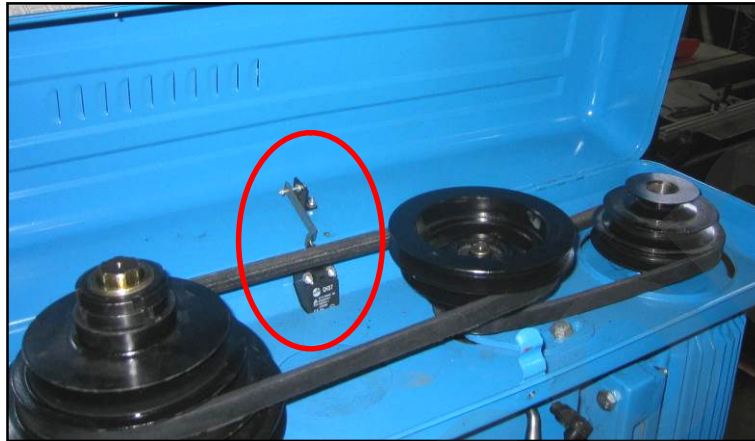
Figure 19 – Guard with micro-switch on the power transmission system.
