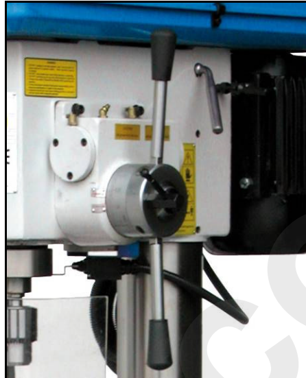
Figure 25 – Installing the handle.
