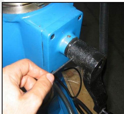
Figure 24 – Dismounting the spindle.
