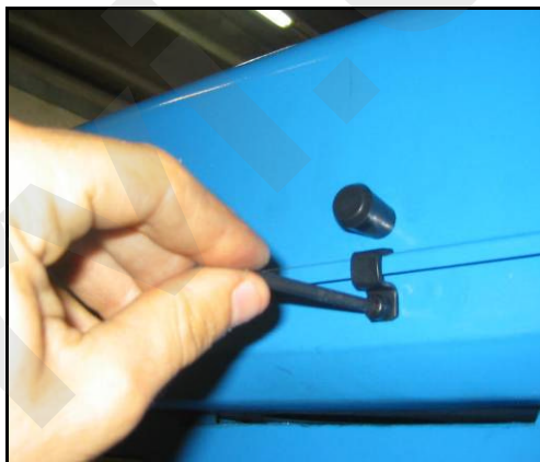
Figure 7 – Undoing the screw of the shield.
