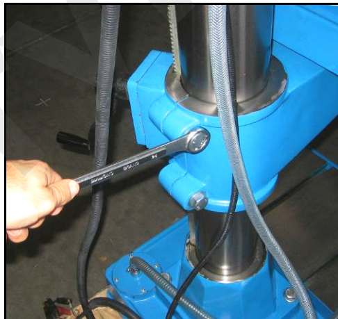
Figure 19 – Unlocking the screws.
