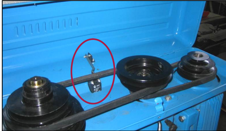
Figure 23 – Guard with micro-switch on the power transmission system.
