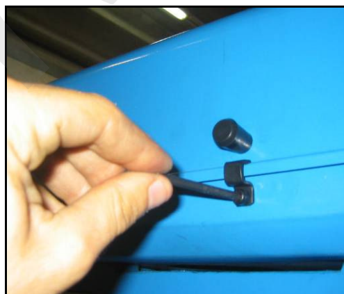
Figure 14 – Undoing the screw of the shield.
