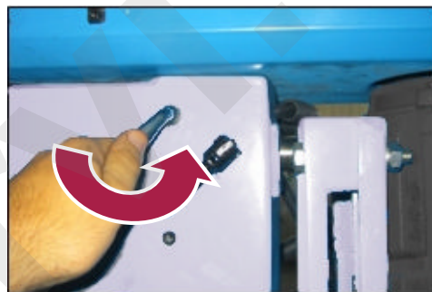
Figure 13 - Loosening the belt tension.
