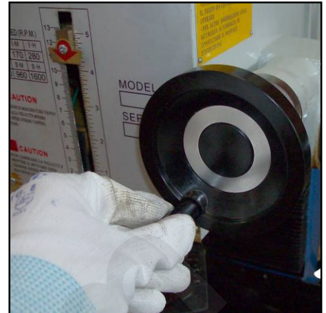
Figure 18 - Hand wheel activation.
