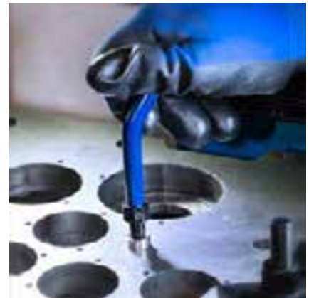
4th operation Screw in the Coil insert with the appropriate tool
