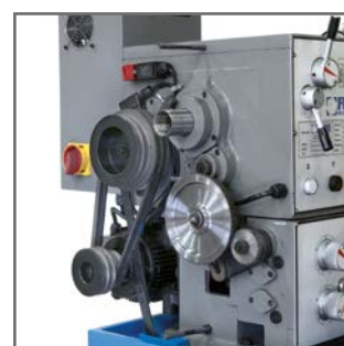
Safety guard with safety micro switch
