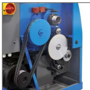
Safety guard with safety micro switch
